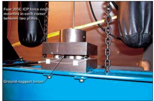
Figure 2. Sensor mounting between two plates (courtesy of Canadian Department of Natural Resources).
