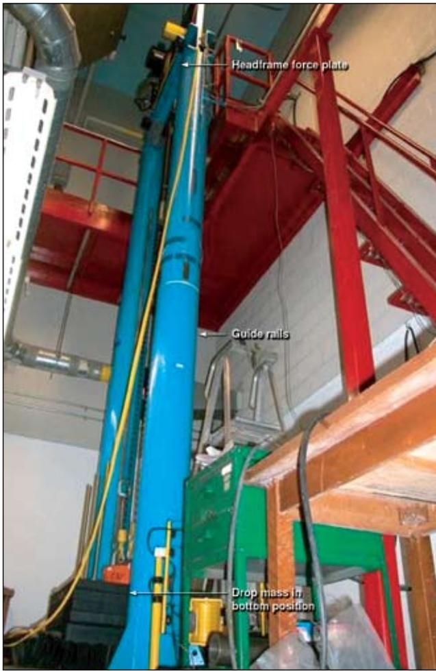
Figure 1. Drop test system (courtesy of Canadian Department of Natural Resources).
