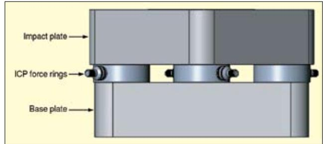
Figure 5. Side view of force plate assembly.
